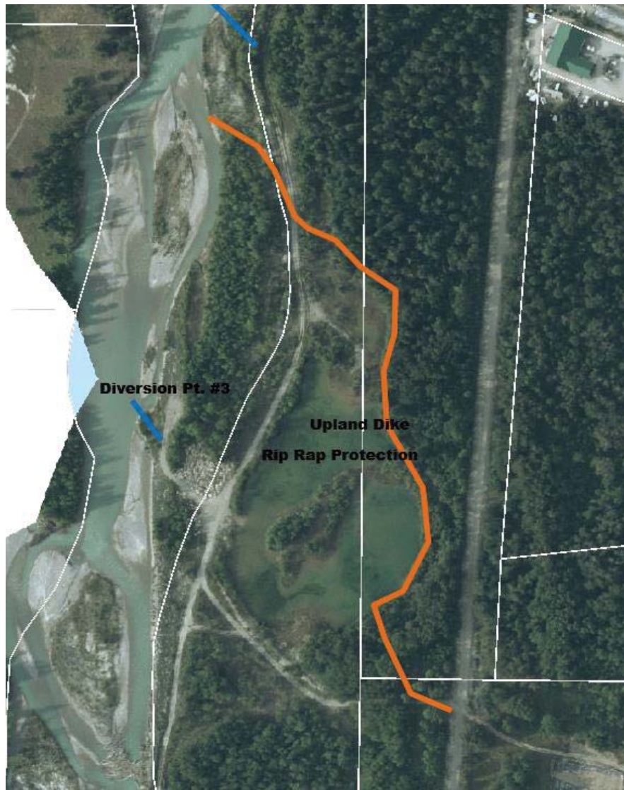
Figure 3. Proposed rip rap armoring in Section 2a, and 3 rd (southern) diversion structure
