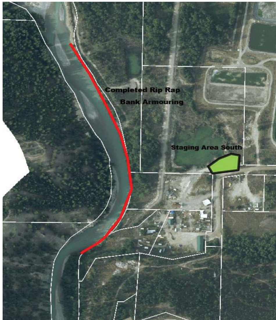
Figure 2. Rip rap armouring already completed and southern marshalling/staging area.
