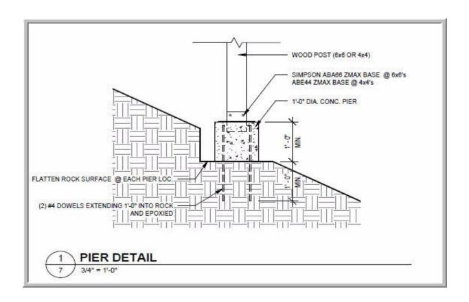
Foundation pier footing detail, which will be imbedded into granite slab with the use of re-bar.
